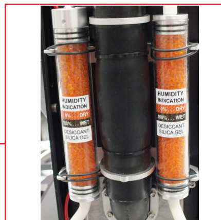
Silica gel desiccants in the fixture arm
