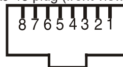
RJ-45 plug (front view):
