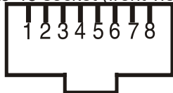
RJ-45 socket (front view):
