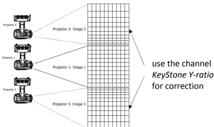
If the channel **Global effect 1 - Parameter 3** is set to the range of 171-180, the aspect ratio of an actual image is displayed in the image. The feature is activated when the Picture Merging is active only.
