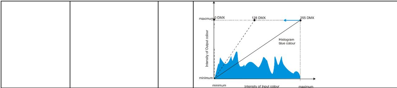
**Brightness scale** (DMX value=69) – the effect changes the output intensity of brightness of the picture.
