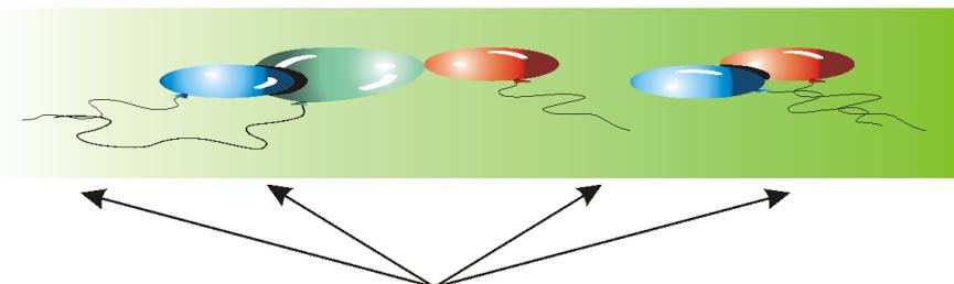
All projected images have resolution 1024 x 768, but the resolution of 1024 pixels is “made ” from 256 pixels as each fixture projects ¼ of the source picture (this quarter has a source resolution 256 x 768).
