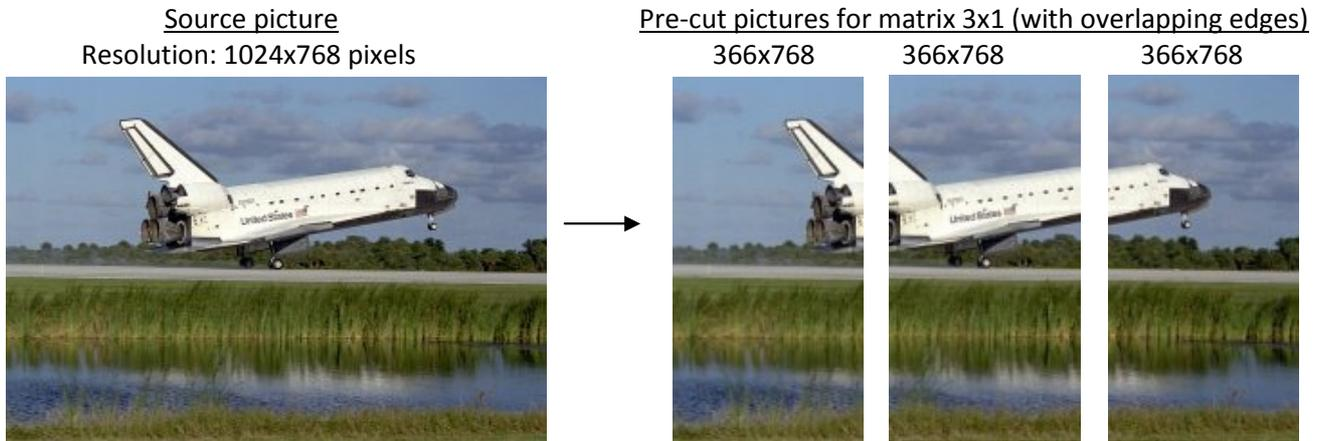
Single segments of the source picture must have the same size (pixels) which is given by:
