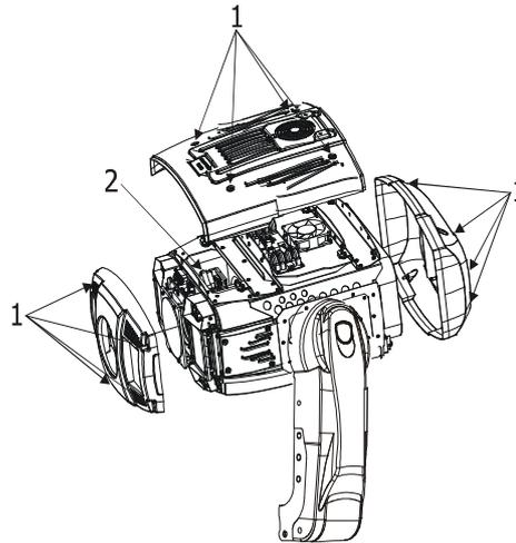
**3.** Unscrew the cable cover (2) and disconnect cables from motors and sensors (3 motor cables and 2 sensor cables) in the front part of the fixture head.
