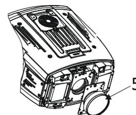
5. Fasten the plastic front cover back on the fixture head by means of the 4 quarter-turn fasteners.
