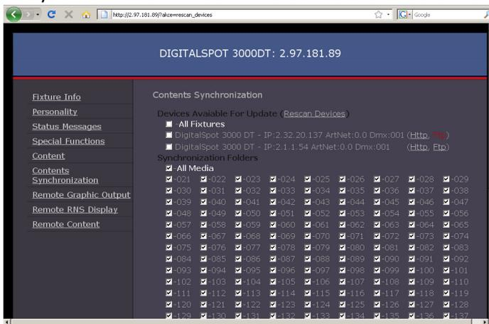
You need to know only IP address of one fixture as the rest of connected fixtures with their IP addresses is displayed in this window. By clicking on the Ftp option (in parenthesis) at desired fixture the FireFTP window will appear:
