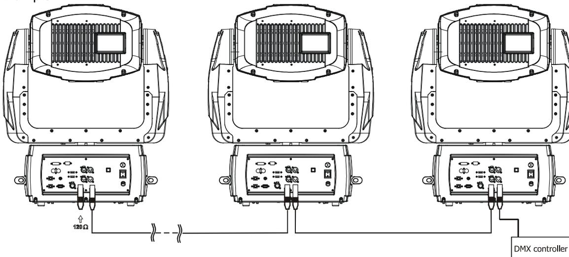
Caution: Terminate the link by installing a termination plug in the DMX output of the last fixture. The termination plug is a male 3-pin XLR plug with a 120 Ohm resistor soldered between Signal (-) and Signal (+).
