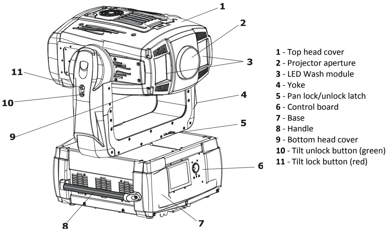
The fixture head is locked for transportation - the tilt lock button (11) is pushed and the pan lock/unlock latch (5) is in a lock position. To unlock the fixture head, press the tilt unlock button (9) and move the pan lock/unlock latch into an unlock position.
