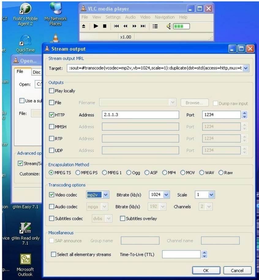
Check the "HTTP" option in a Outputs column, type an IP address of the PC in the "Address" field and a figure port in the "port" field.
