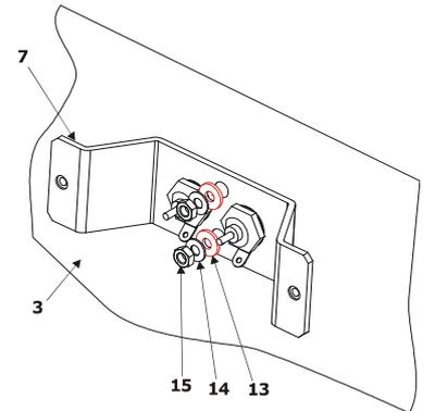
**Warning:** The SDI/ASI connectors holder has to be electrically insulated from the rear panel otherwise the capture card can be damaged.
