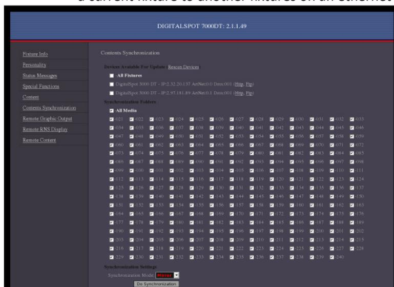
There is a list of available fixtures under **Device Available for Update**. If you connect another fixture to a network, use option "**Rescan Devices**" to refresh the list of fixtures.
