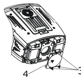
4. Place the long (short) throw optic module (5) instead of the module of the glass cover (4) and secure it by the 3 quarter-turn fasteners (6).
