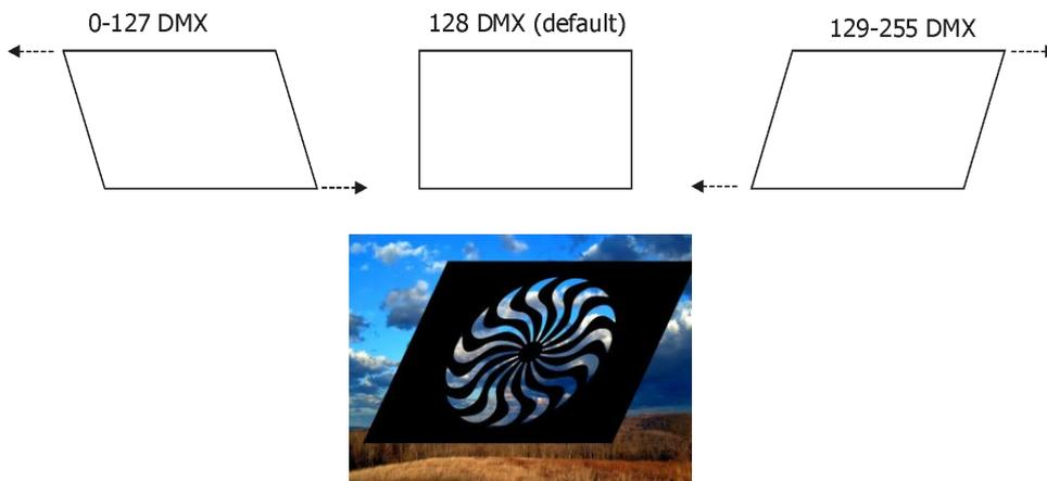
The channel **Gobo effect 1 – Parameter 2** skews the image in Y-axis.
