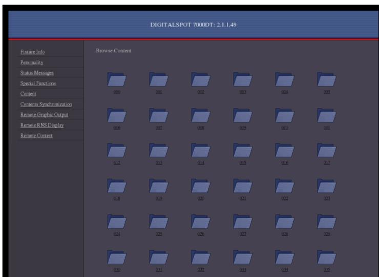
**Contents Synchronization** - the window allows you copy (addition) media content from a current fixture to another fixtures on an ethernet network.
