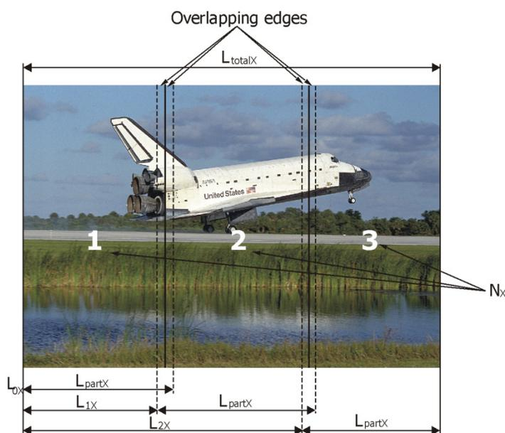
Size of segments in X-axis:  $L_{partX} = L_{totalX} / [x - (b/100) * (x-1)]$
