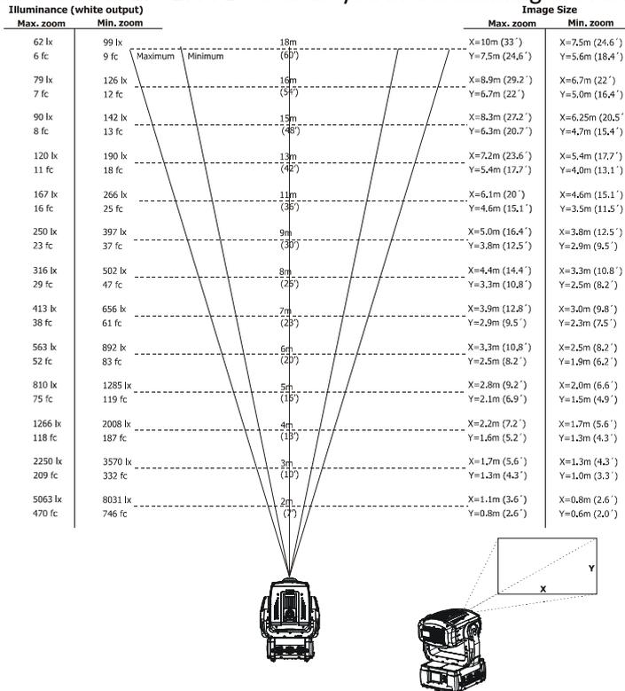
**Note:** There is a tolerance among these numbers due to optical component variations. We recommend that if you intend to permanently install the DigitalSpot 7000 DT, you should physically test the projection size and distance
