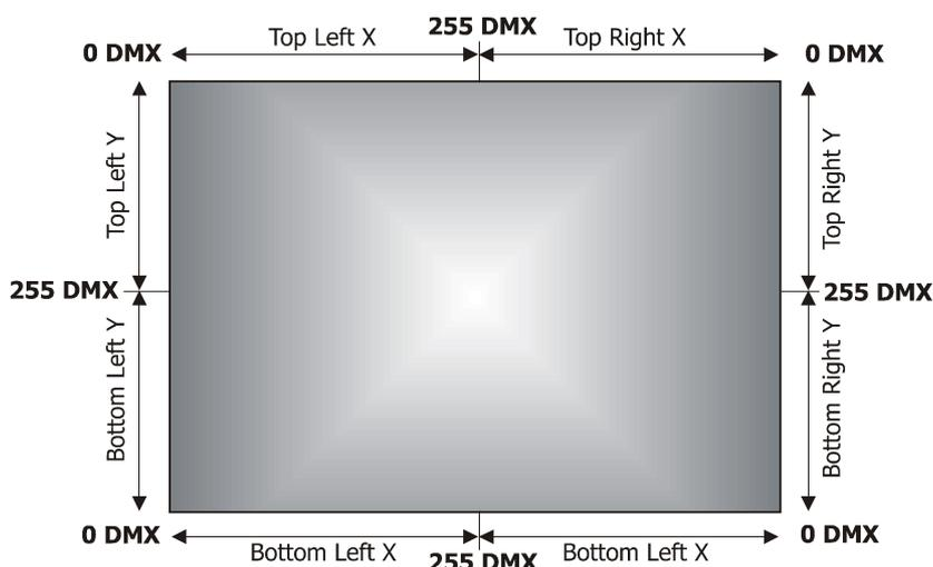
Setting all keystone values to 0 will place all four corners of the image at the four corners of the projector output. The keystone values can also be used to create interesting skewing effects.
