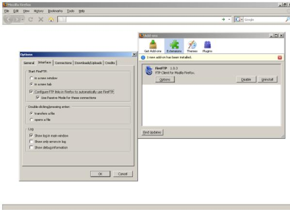
After installing FTP client, run Mozilla Firefox and type the IP address of desired fixture in ftp format e. g. **ftp://2.97.181.89** and a Fire FTP window will appear.
