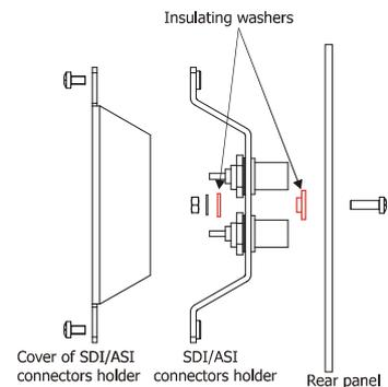
7. Screw the cover (7) to the SDI/ASI connectors holder (8) with two screws M3x6 (9). Screw the rear panel (3) back to the chassis.
