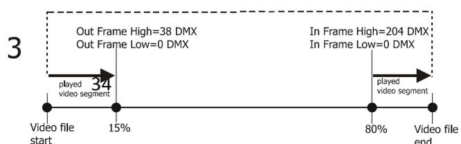
3. It is possible to skip a segment in the video file by setting the In Frame to a point following the Out Frame value.
