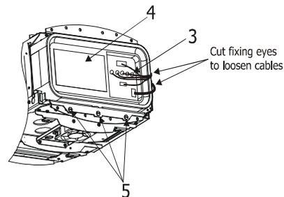
**5.** Unscrew the two Allen screws (5) at the bottom part of the projector chassis (7).
