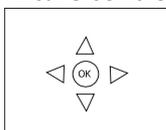
The [RNS] encoder wheel controls movement between arrow fields on the control display and the [ENTER] button enables movement in menu. Pressing the [ENTER] on a circular field (marked "OK") confirms selected options. The [ESC] button leaves menu without saving changes.
