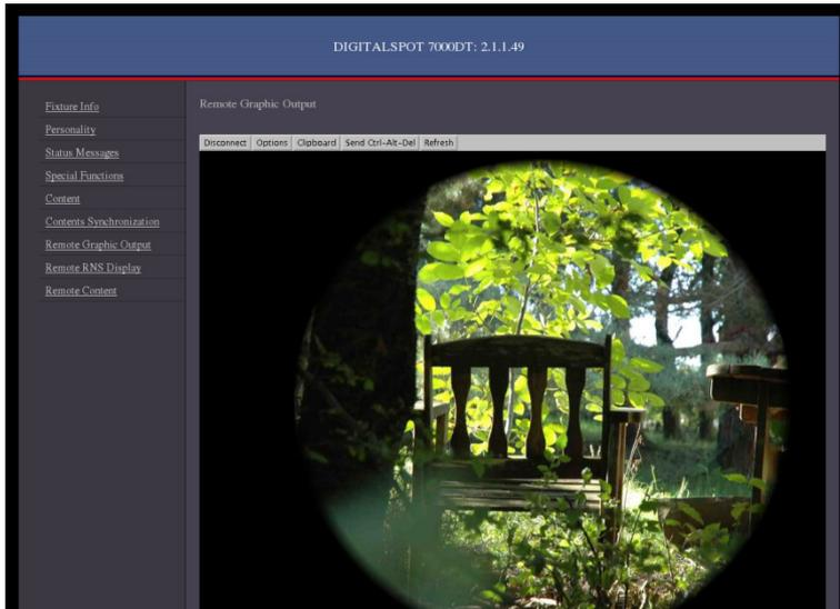
**Remote RNS Display** - the window "takes" the fixture's control panel. You can browse and adjust all items in this fixture menu by means of your keyboard. Use the Up/Down and Enter/Escape keys.
