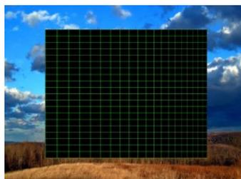
The channel **Gobo effect 2 – Parameter 3** compresses or expands the image in Y- axis.
