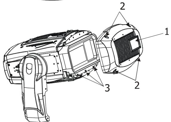
**5** Loosen the screw and open the lamp cover. Pull out the lamp by using the built in handle. Do not turn the power on with the lamp cover removed.
