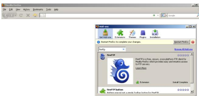
5. After installation, go to the “ Tools”, select “Add-ons” item, select “Extensions” in the toolbar and click on the Options button. Select “Interface” menu and check option “**Configure FTP links in Firefox to automatically use FireFTP**”.
