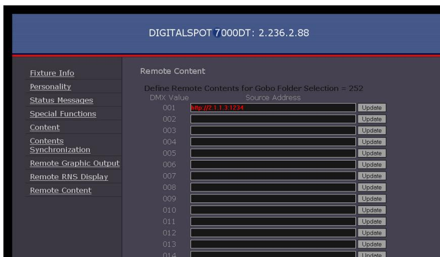
Type in the "source Address" field the IP address and the port number of the streaming source (in our case it is a PC) in this format: http://2.x.x.x:port number e.g. http://2.1.1.3:1234 and save it by clicking the "Update" button. This way defined streaming source is assigned to a DMX value of 1 at the channel **Gobo selection**.
