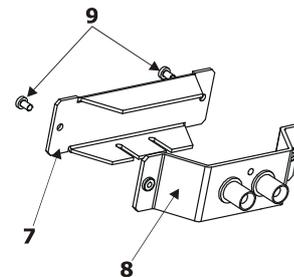
6. Snap the two insulating washers with outer diameter of 10mm (10) into SDI/ASI connectors holder (8) and fasten this holder on the rear panel (3) with two screws M3x10 (9). The SDI/ASI cables (11) have to aim at the bottom of the fixture base.
