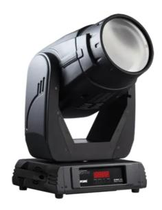
The ROBIN 300E Beam Classic has a colour wheel with 7 replaceable 'Slot&Lock' dichroic filters, plus both static and rotating gobo wheels. A variable frost effect ensures a smooth transition from a beam light to a regular wash light, and there is also full dimming, variable strobe effect and pan/tilt of 540/260 degrees.
